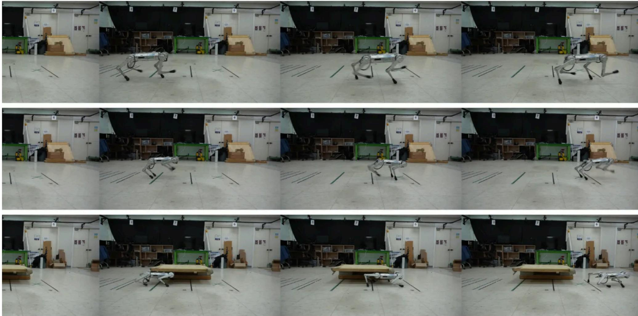
d experiments of generating multiple motions by varying constraints. A robot walking with a trotting gait (top) was changed to locomote gait (middle) or crawl beneath an overhanging obstacle (bottom) by modifying the gait pattern constraint or COM height with joint angle
